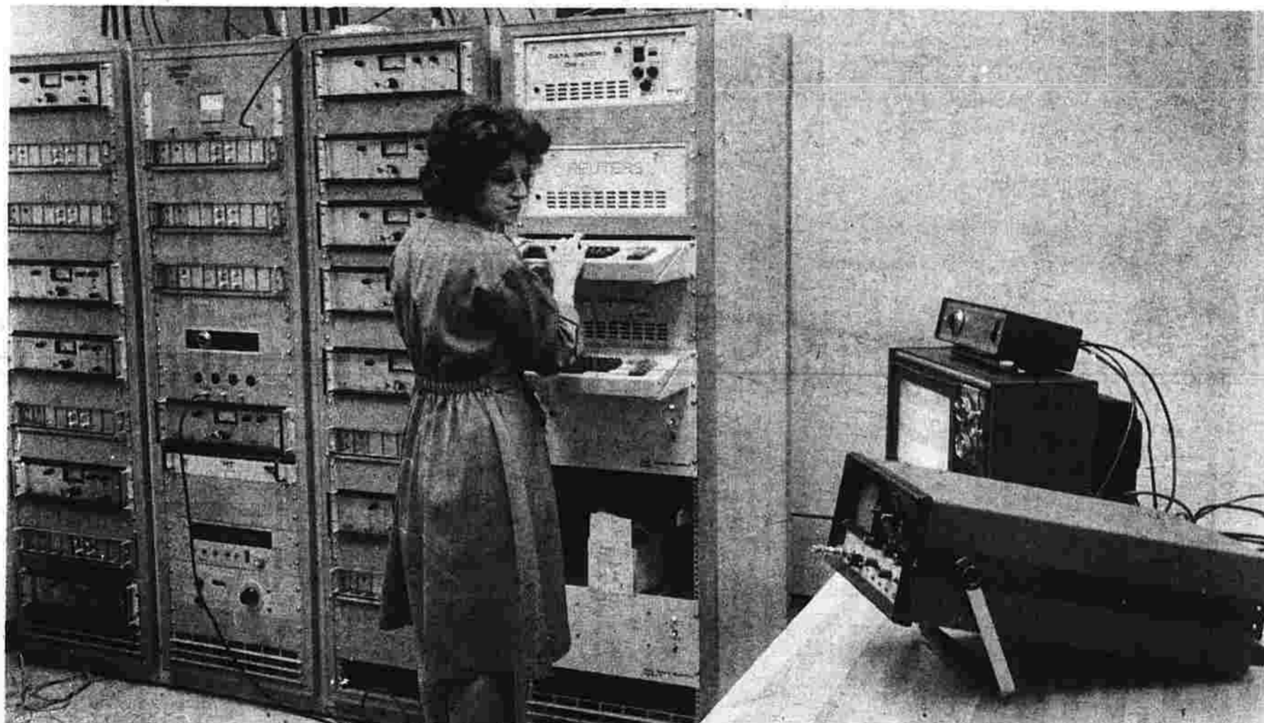
Michele Gorra-O'Neil of Vernon programs one of cable television's four automated information channels, which run 24 hours a day. She's using a keyboard terminal similar to that used in computers to type in news of upcoming TV programs. The four channels are TV guide, news, weather, and sports/financial.
